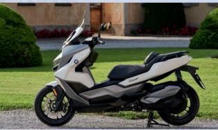
front discs with radial 28mm single piston floating calipers and the braking system included a Continental MK 100 MAB 2-channel ABS unit allowing independent control of the front and rear wheel circuits. As on the C650, the geometry and feel were designed to replicate motorcycle characteristics. The C400GT joined the C400X for 2019, this offering increased comfort and touring capability.
